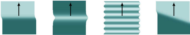
Fig. 2.5 Planar waves: front, pulse, periodic wave, and a rotated front (from left to the right). The arrows indicate the direction of propagation y .
